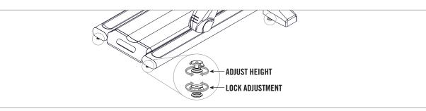
E) Adjust the **2 REAR LEVELERS** so the elliptical is level on the floor. Then adjust the 2 MIDDLE STABILIZER CAP LEVELERS so they are snug with the floor.
