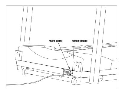
Connect power plug to the treadmill and connect the cord to a power outlet. The on/off switch is located next to the power cord. Flip this switch to the 'ON' position, so that the switch is lit. You will hear a beep and the console will light up.
