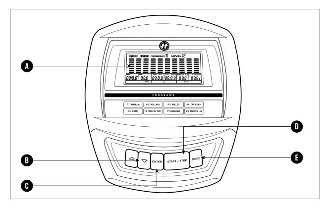
*Note:* There is a thin protective sheet of clear plastic on the overlay of the console and should be removed. *A) MONITOR DISPLAY:* Start, Stop, Program Profile, Level, Time, MPH, RPM, Distance, ODO, Calories, Watts, Age, Target H.R., and Heart Rate.
