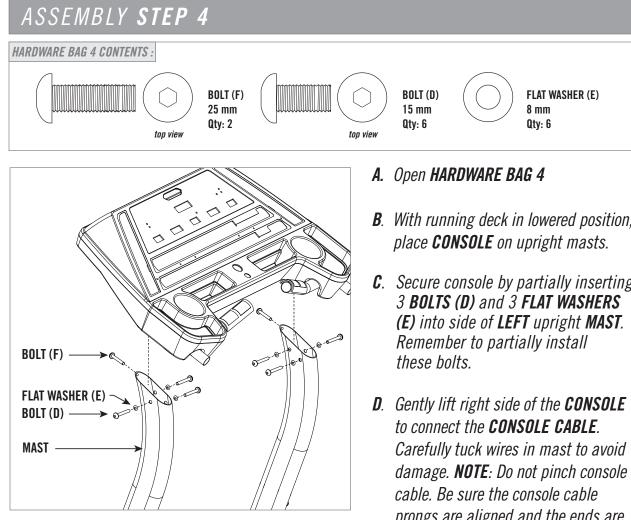
\* Be sure to tighten bolts after all are lined up.
