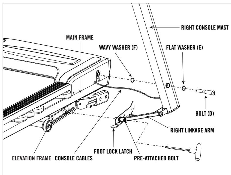
**A** Pull **LEAD WIRE** through **RIGHT CONSOLE MAST**. After pulling the **LEAD WIRE** through the mast, the top of the **CONSOLE CABLES** should be located at the top of the mast. Detach and discard **LEAD WIRE**.
