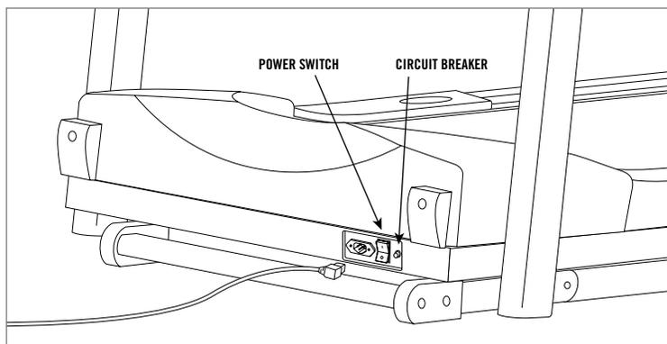
Connect power plug to the treadmill and connect the cord to a power outlet. The on/off switch is located next to the power cord. Flip this switch to the 'ON' position, so that the switch is lit. You will hear a beep and the console will turn on.
