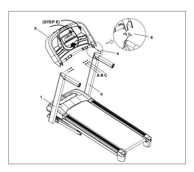
NOTE: Be careful not to pinch any wires while assembling the console.
