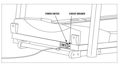
Connect power plug to the treadmill and connect the cord to a power outlet. The on/off switch is located next to the power cord. Flip this switch to the 'ON' position, so that the switch is lit. You will hear a beep and the console will light up.
