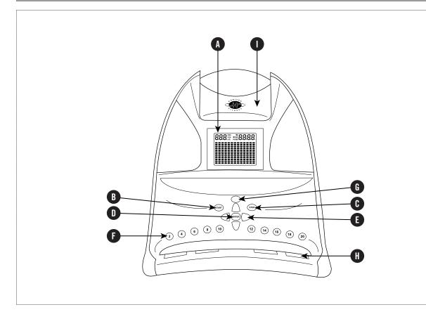
A) MONITOR DISPLAY: Speed, Time, Pulse, Distance, Level, Calories and Program Profiles.
