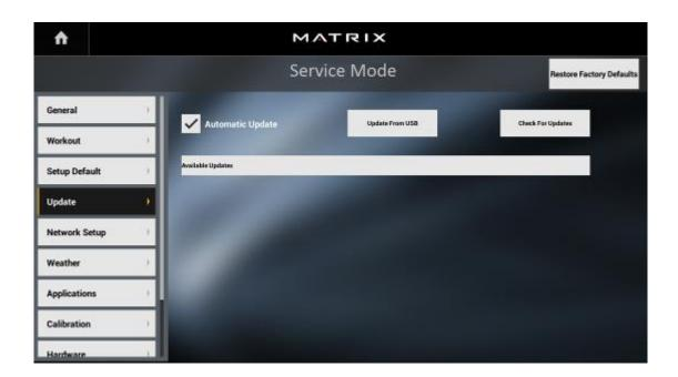
Insert well-prepared USB flash driver into console USB, select "automatic update", software can be updated.
