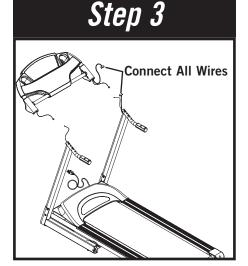
1. Connect both pulse grip and console mast wires. Carefully tuck wires in mast to avoid damage. NOTE: Do not pinch wires
