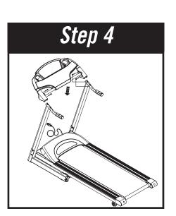
**1.** Attach the console to the pulse grips. Again, carefully tuck all wires in mast to avoid damage.
