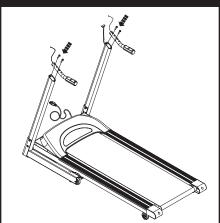
Place pulse grip handlebars to its correct position.
