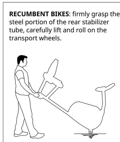
**RECUMBENT BIKES:** firmly grasp the steel portion of the rear stabilizer tube, carefully lift and roll on the transport wheels.
