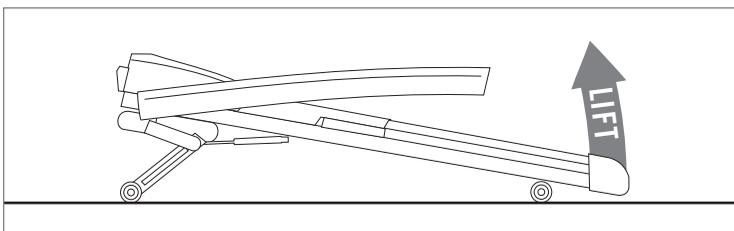
**PROBLEM:** The banding straps were removed before **ASSEMBLY STEP 1** was complete and the machine has sprung open and cannot be assembled.
