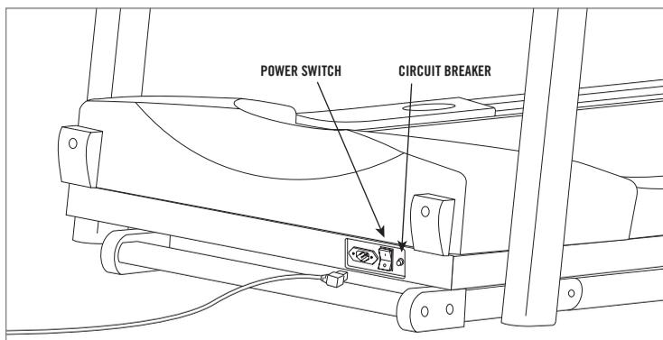
Connect power plug to the treadmill and connect the cord to a power outlet. The on/off switch is located next to the power cord. Flip this switch to the 'on' position, so that the switch is lit. You will hear a beep and the console will light up.
