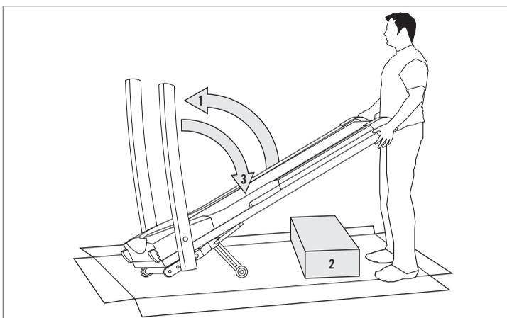
**F** Lift the **RUNNING DECK** until lock latch on side of treadmill is fully engaged.
