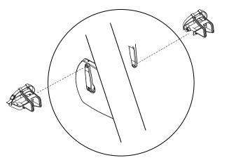
A Install the pedals on the pedal cranks by using the Open Wrench (Z32). The closed end of the pedal cage must point forward, toward the front of the cycle.
