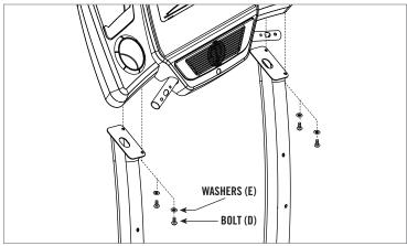
\* Be sure to tighten bolts after all are lined up.
