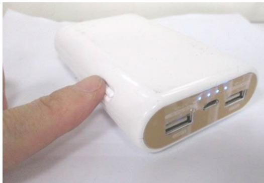
To check the charge of a battery, press the button on the side. Each of the 4 LEDs that illuminate describe 25% or maximum charge.
