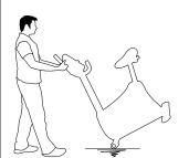
**RECUMBENT BIKES:** firmly grasp the steel portion of the rear stabilizer tube, carefully lift and roll on the transport wheels.
