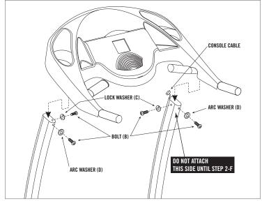
\* Be sure to tighten bolts after all are lined up.
